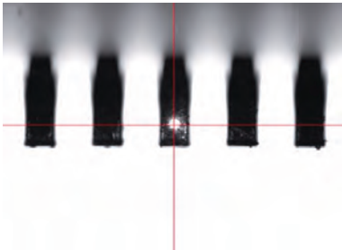
Laser spot of Tracking Auto Focus system (TAF)
