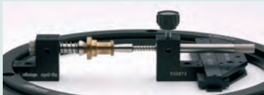
Holding a cylindrical part between clamping tips.
