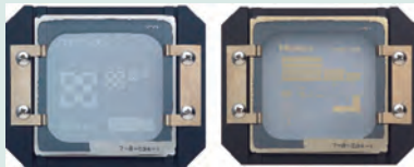
Calibration Glass chart & Compensation glass chart with holder
