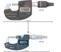
Comparative sizes: High Accuracy-Micrometer with a highly rigid frame and a common Micrometer with a standard frame
