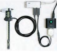
Sample application with USB Input Tool Direct
