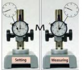
Should the workpiece be approx. 1 mm larger than the nominal dimension, the part is assessed as good if the smaller pointer is ignored.
