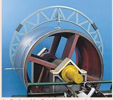
Application with adjustable stop on workpiece
